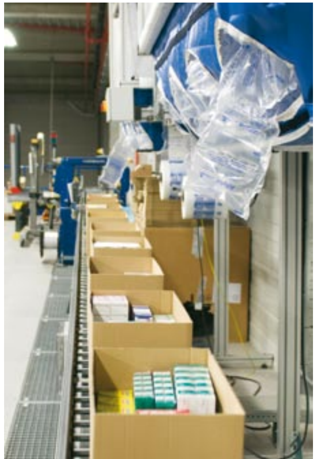
AIRplus® machines keep packing materials readily available by continually filling multiple access storage bins over packaging stations.
