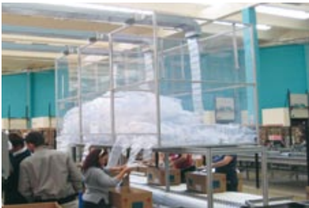
AIRplus® integrated systems continually feed air bags into bins over the packing station for quick and convenient access.
